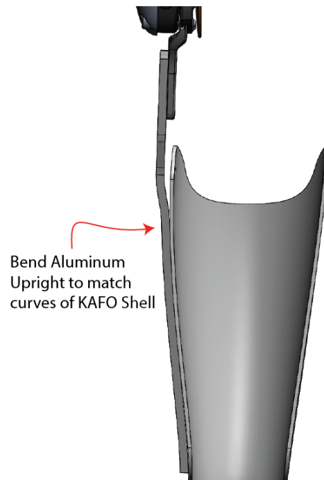
Figure 14 Bending Aluminum Upright
